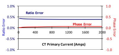
CT testing performed with 16" RoCoil. Conductor used filled 90% of RoCoil window.
