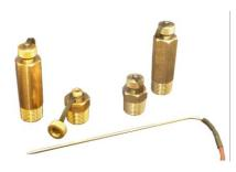
The "Test Plugs" probe, also called "binder probes", offers an excellent solution to get high accuracy and quick response as the sensor is inserted in the flow. They eliminate the temperature pockets that delay response and create a risk for freezing at low temperature and the sensors can easily be removed for calibration. Type C - Probe is 150 mm long with 3 mm diameter with an angle to give a good hold when it is inserted or removed.
