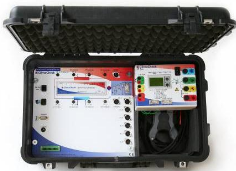
Figure 1, Field kit for Performance Inspection technology that does not require installation of flow meters to establish the performance and capacity.
