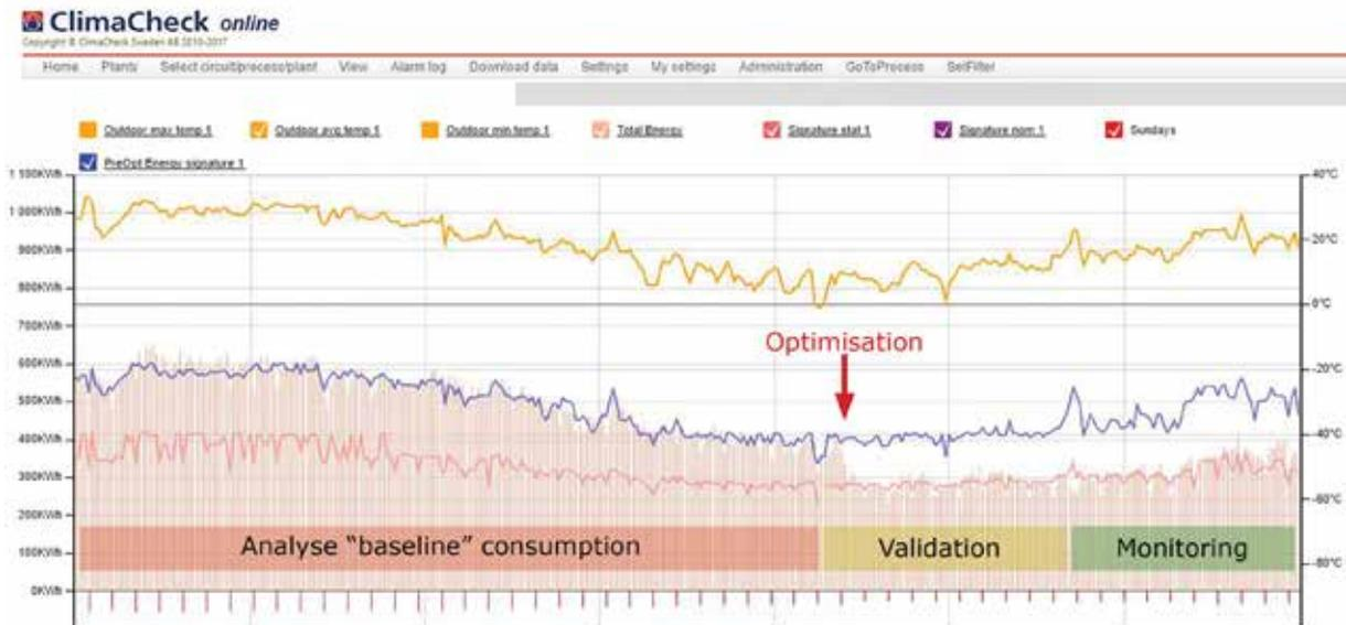
**ClimaCheck online** makes it possible to monitor your HVACR-system and to apply energy optimisation and preventive maintenance, which normally leads to 10-30% energy savings. It is also possible to receive early text/email warnings if the system's energy signature is changing, and allowing you to fix problems before a breakdown.
