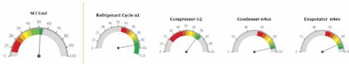
**SEI - System Efficiency Index** and the sub-efficiencies for the main components are powerful tools developed by ClimaCheck, test Institutes and trade organisations in Europe to visualise performance for operational staff, maintenance technicians and engineers. The conventional indicators kW per RT, COP or EER do not give reliable information in the field where systems often operate far from rated performance.
