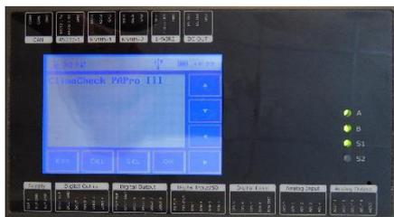
This enables integration with building management systems (BMS) and allows them to write measurement inputs to the PA Pro III and read back calculated results such as COP and System Efficiency Index.
