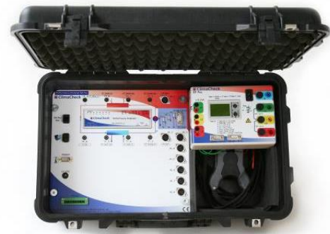
Figure 4, Field kit for Performance Analyser that does not require installation of flow meters to establish the performance and capacity.
